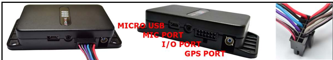
Figure 2 - T23 FLEET I/O PORT & I/O CABLE
