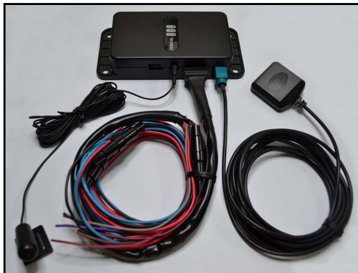
Figure 4 - T23 FLEET Automotive Installation/Wires Connected
