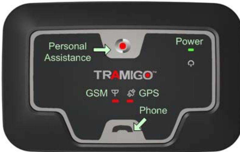
Figure 1 - T22 Unit Controls
