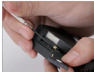
Removing the SIM holder.
